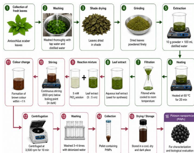
Figure 1 Schematic illustration of synthesized PtNPs using Anisochilus scaber Benth leaf extract
