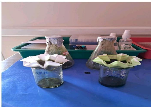
Fig 1b: Figure: Filtration of the solvent extract
