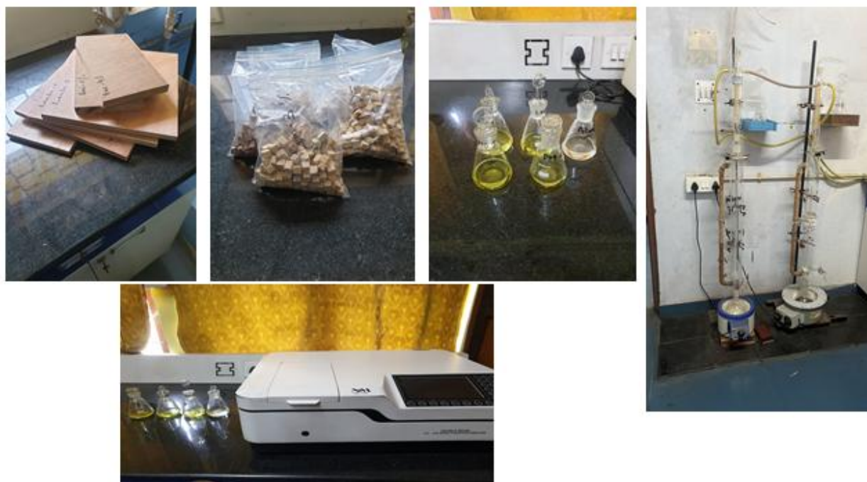
Figure 3. Testing of formaldehyde content as per IS 13745
