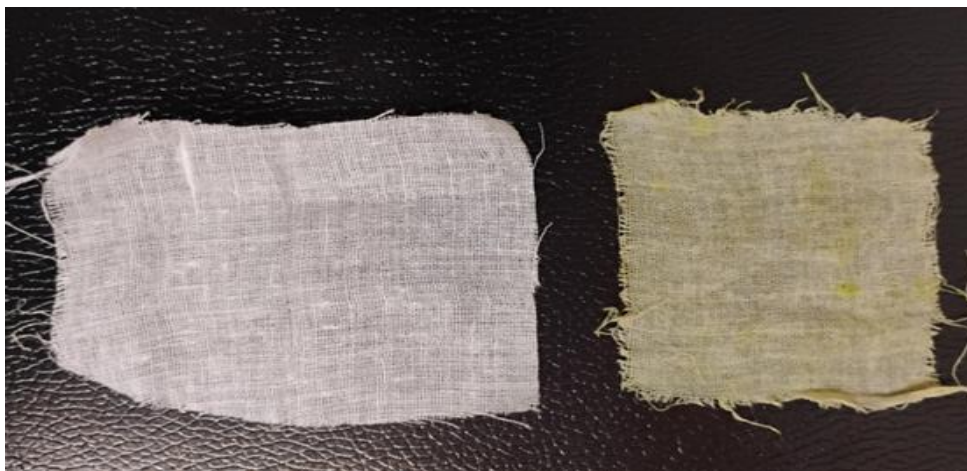
Figure 3.7: Application of extracted pigment of WS2 on to white colored cotton cloth turn slight green
