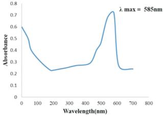
Figure 1.UV-Vis absorption spectrum of C. Annuum synthesized CuNPs
