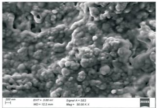
Figure 4. SEM image of synthesized CuNPs
