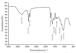
Figure 2. FTIR spectra of biosynthesized copper nanoparticles
