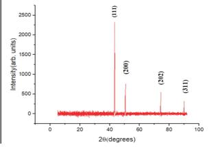
Figure 3. XRD analysis of copper nanoparticles
